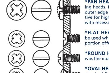
\*PAN HEAD: Recommended for new designs to replace round, truss and binding heads. Provides a low large diameter head, but with characteristically high outer edge along the periphery of the head where driving action is most effective for high tightening torques. Slightly different head contour where supplied with recessed head. See dotted line.
