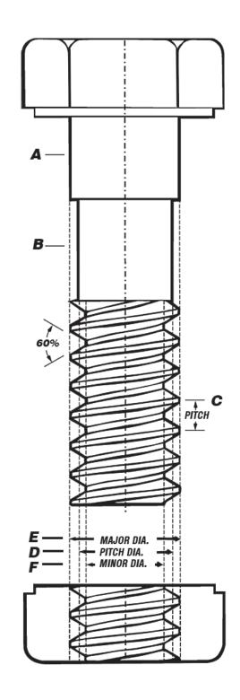
**A. FULL DIAMETER SHANK:** Equal to major diameter of thread. Produced by cut thread or by roll thread on extruded blank. Characteristic of machine bolts and cap screws.
